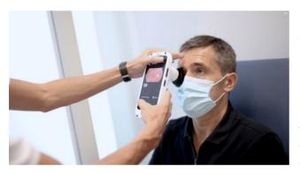
The Retina Read Risk solution (represented on the left) consists in: (i) a device, containing a lens, which is placed on a smartphone camera, to capture the fundus images, (ii) a program to define a patient profile and (iii) an application with an AI for analysis.
